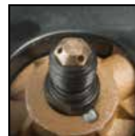
Through the spindle water spray for even dispersal
