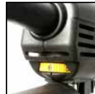
Variable speed for control of material removal rate
