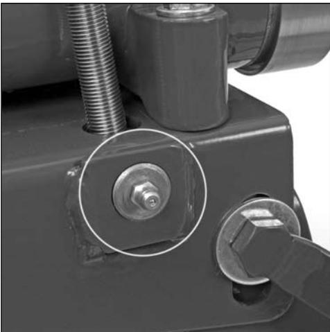
*Grinding head external zerk fitting*
